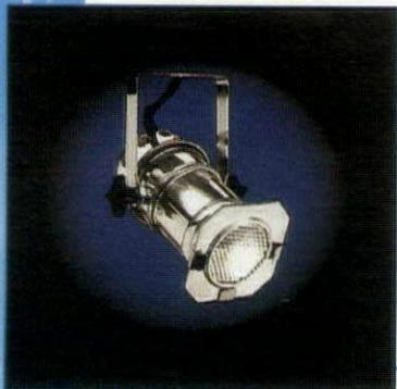
The new L1816 lampholder from **Cooper Lighting's Halo** is scaled for use with 75W MR16 sources on Halo Power Trac and Lazer-by-Halo track systems. A die-formed aluminum yoke allows the lampholder to rotate horizontally 338 degrees and adjust 0-90 degrees vertically. Available in polished aluminum, matte black and white, the lampholder includes an integral 12V electronic transformer that features a visual polarity line for proper grounding when attaching to track systems. **Circle No. 124**
