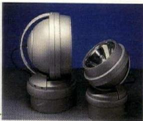
Available in small (OS) and large (OL) models, **Architectural Area Lighting's** Oculus utilizes a parabolic reflector system and axial lamp orientation to provide beam control and reduce glare. Suited for wall-, ceiling-, pole- and floor-mounting configurations in interior and exterior settings, Oculus comes in metal halide, compact fluorescent and PAR lamp versions. T6 ceramic lamp models as well as various internal and external options are offered. **Circle No. 189**
