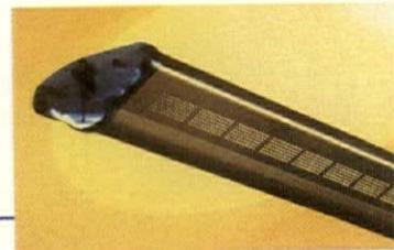
Venza LP from **Ledalite** is offered in a one- or two-T8-lamp version and a T5/HO version. Venza offers semi-indirect, indirect and wall-mounted distributions and is available in 4-ft., 8-ft. and 12-ft. lengths. Housing is die-formed, 20-gauge cold-rolled steel. Finish is standard white or Techspace natural steel metallic powder coat. Translucent endcaps come in seven colors. UL-listed. **Circle No. 167**
