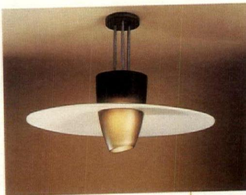
Designed by Adam D. Tihany for **Sirmos**, the Amp-Rex pendant sports a canopy and body core formed of CyTron translucent resin and suspended by a trio of brushed nickel rods. The fixture has a 32-in. diameter, 12<sup>1</sup>/<sub>2</sub>-in. depth and a 24-in. drop. Providing both direct and indirect lighting, the fixture is lamped with a 60W Edison-type, medium-base incandescent source. A selection of finishes is offered, including onyx-whitehaze (shown). **Circle No. 91**
