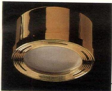
Specialty Lighting's Lovo/Lux recessed and surface-mounted accent lighting fixtures are available individually or in sets of two, three or six. Housings measure 2 9/16 in. in diameter and are offered in polished brass, polished chrome, matte black or matte white finishes. Press-in side tabs facilitate recess mounting and attached 7/8-in.-deep saucer cups enable surface mounting. Lovo/Lux accepts 10W and 20W T2 bi-pin halogen lamps. **Circle No. 155**
