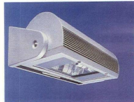
The WFL series of architectural wall-mounted fixtures from **Lithonia Lighting** offers a choice of 10 different optics and a range of rotation and reversible-mounting capabilities in either lens-up or lens-down configurations. In the down configuration, full cutoff lighting meets IES criteria. Construction consists of a cast and extruded aluminum housing and a one-piece silicone gasket. The series accommodates metal halide and HPS lamps. **Circle No. 179**
