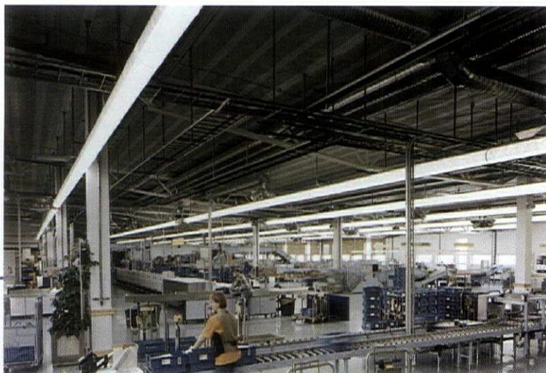
LIGHT PIPE INSTALLATIONS SUCH AS THIS ONE, A MANUFACTURING FACILITY, RESULTED IN INCREASED LIGHT LEVELS. HERE, LIGHT PIPE REPLACED METAL HALIDE DOWNLIGHTS.
