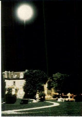
**SOLARC, A TETHERED HELIUM-FILLED BALLOON FITTED WITH METAL HALIDE LAMPS, BLANKETS THIS LARGE OUTDOOR AREA WITH LIGHT.**
