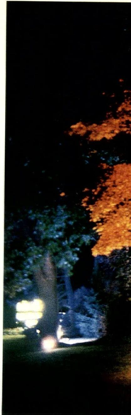
**SPRUCING UP:** Bowden Square's Colorado Blue Spruce (top left) is lit in front with a dichro blue filtered lamp and from behind with a 90-watt VNSP to produce a moonlighting effect. The auburn hues of the Japanese Red Maple are emphasized with 150-watt dichroic filtered lamps (above & left).
