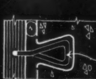
Cramp and S-hook into pocket left by contractor
