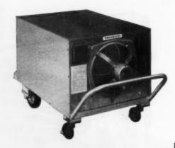
Totally enclosed fan draws in cold damp air. Moisture condenses on the evaporator coils. Cold dry air passes over condenser thus raising air temperature.
