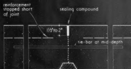
fracturing controlled by slot and batten
