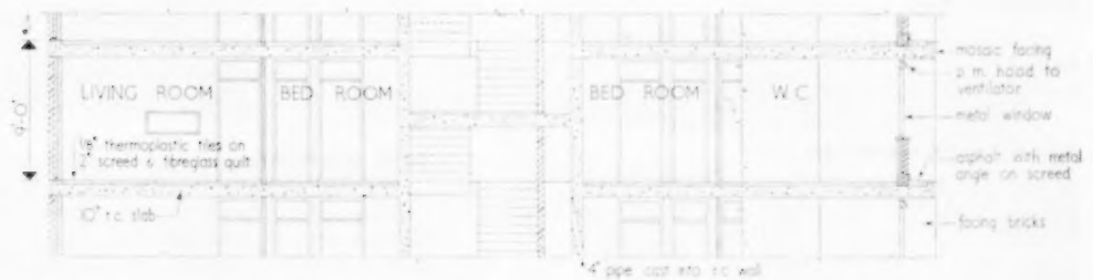
Section through typical floor in tower block
