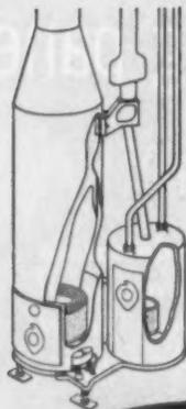
The BAXI-OIL '40', showing air heat exchanger with independent high-efficiency domestic water heater. Also available: the BAXI-OIL '32', without water heater.
