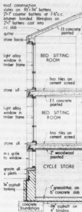
Section through external wall [Scale 1/4 in. = 1 ft. 0 in.]
