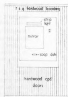
Section and elevation of washbasin-unit [Scale: 1/4" = 1' 0"]
