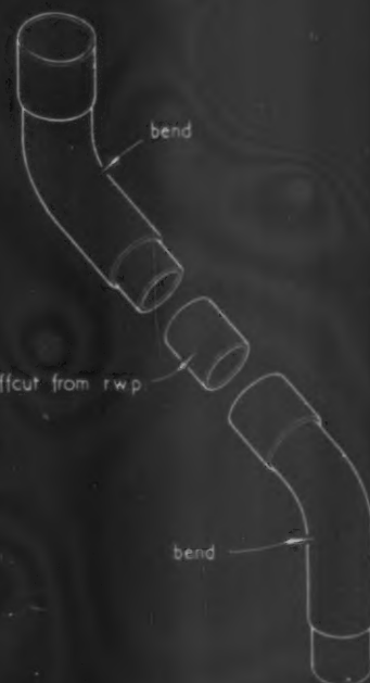
METHOD OF FORMING OFFSETS FOR 3 1/2", 4" AND 6" PIPES
