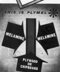
W.C. Compartments and shower cubicles in Plymel, the new melamine-faced material by Venesta Limited, are prefabricated in standard units to save hours of your time.
