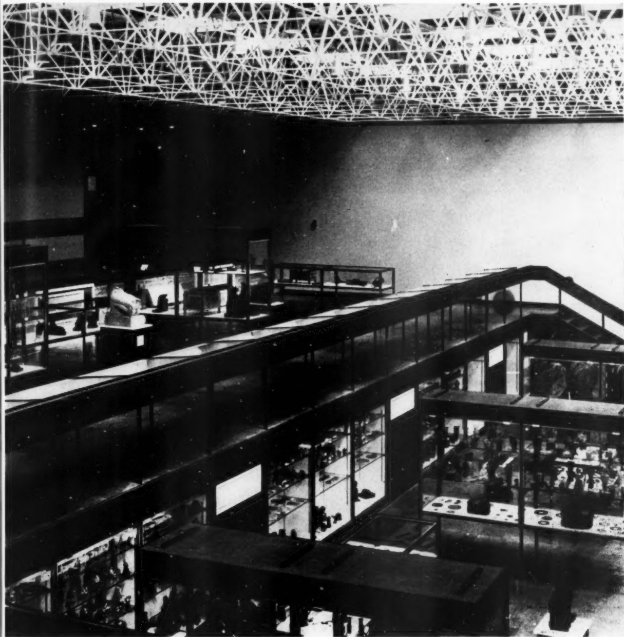
View across the museum to the entrance. The blank panels with louvres contain the heating system. The roof, despite its apparent complexity, is not oppressive or distracting, although the coloured light fittings compete rather unfortunately with the structure.
