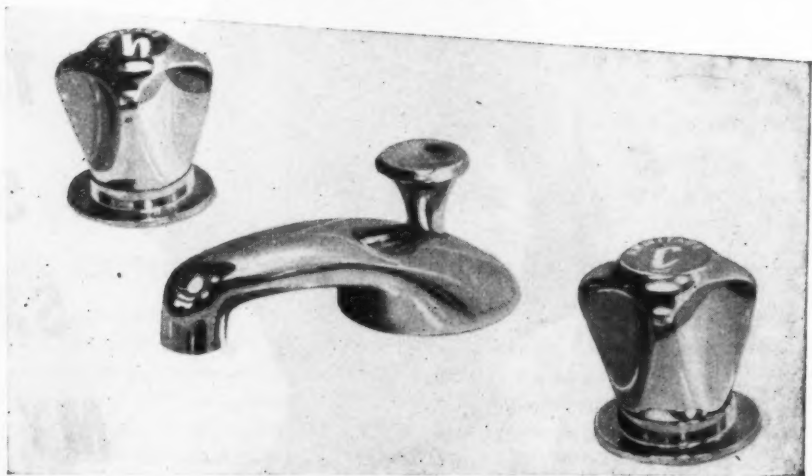
G1050 \frac{1}{2} " Washbasin mixer fitting with 1\frac{1}{4} " pop-up waste. Inlets screwed \frac{1}{2} " B.S. pipe, male, with centres 8" to 10". A truly serviceable and attractive adjunct to any modern bathroom.
