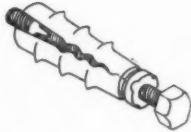
Fig. 7. Non-adjustable attachments to concrete.
