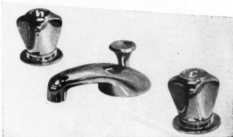
G1050 \frac{1}{2} " Washbasin mixer fitting with 1\frac{1}{2} " pop-up waste. Inlets screwed \frac{1}{2} " B.S. pipe, male, with centres 8" to 10". A truly serviceable and attractive adjunct to any modern bathroom.
