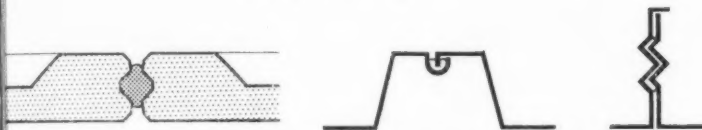
Fig. 8. Protection of mastic joint by reducing area of exposure.
