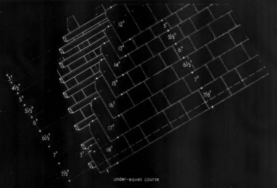
ISOMETRIC VIEW OF TYPICAL RANDOM SLATING. (laid to 3"min. lap)
