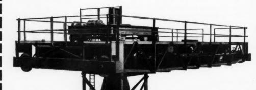
This specially designed Electric Overhead Travelling Crane has an underslung jib which revolves in a complete circle, thus giving maximum hook coverage over the floor area, and also enabling loads to be transferred to adjacent bays. The positioning of the controls gives the operator an excellent view of the load. This crane is another example of the flexibility of our design. When you have a lifting problemcall in John Smiths!
