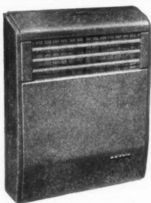
Type 'WM' wall-mounting Thermovent heater. 1\frac{1}{2} and 2\frac{1}{2} kW loadings. Robust welded sheet steel construction with light 'hammered bronze' stove enamel finish.
