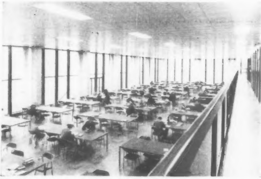
The main reading room from the upper tier of the open access stack. White painted heated ceiling. Grey lino floor. Mullions painted dark blue grey standing on noir vein marble sill. Aluminium column cladding cellulosed aluminium colour. Table tops and chair seats in black leather cloth. White curtains.
