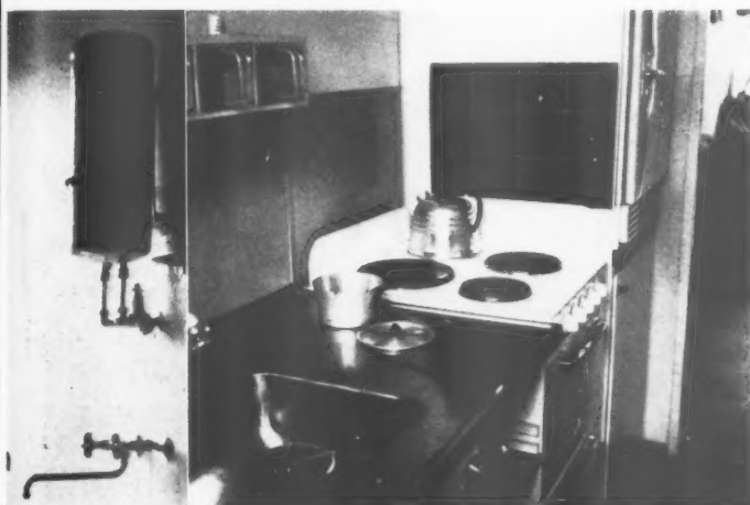
Above right, a typical kitchen in the Hansa Quarter showing the double stainless steel sink, electric cooker and refrigerator. The flats are "all electric," no gas being laid on in this area. Refrigerators are built in and paid for as an addition to the rent. Very few flats have separate ventilated larders as required in this country although we did see relatively small ventilated cupboards (about 2 ft. square) in the social housing projects. Above left, an instantaneous electric water heater of a type not used here. Water softening plants are installed in some blocks, which would overcome a possible loss of efficiency if this type of heater were used with "hard" water.
