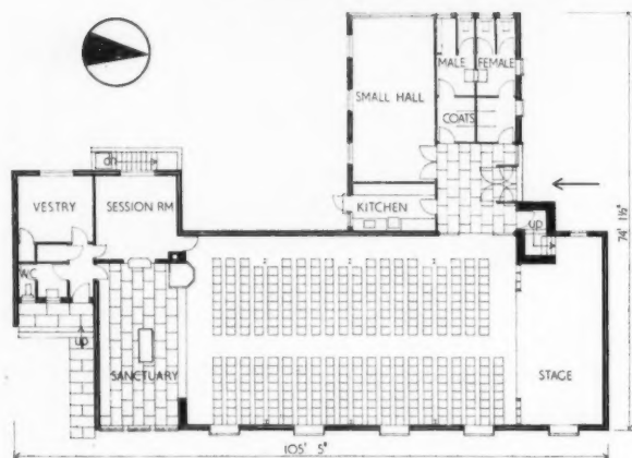
Ground floor plan, Easthouses Church [Scale: \frac{1}{8}" = 1' 0" ]
