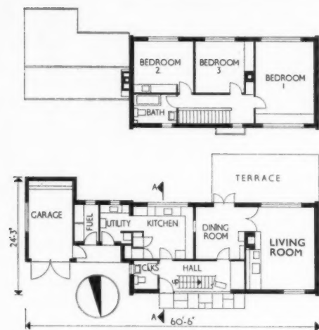
Ground and first floor plans [Scale: \frac{1}{8}'' = 1' 0'' ]
