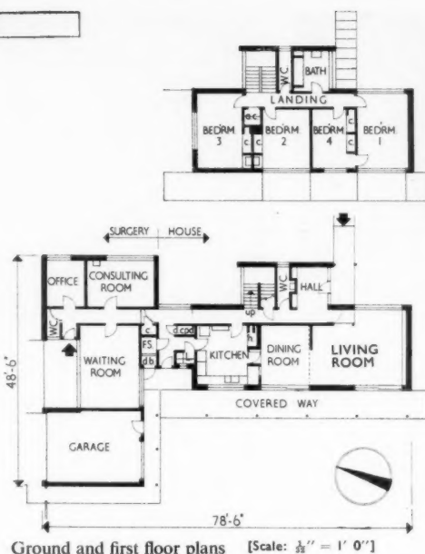
Ground and first floor plans [Scale: \frac{1}{8}'' = 1' 0'' ]
