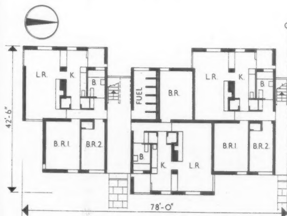
Ground floor plan, Block 1 [Scale: \frac{3}{8} " = 1' 0"]
