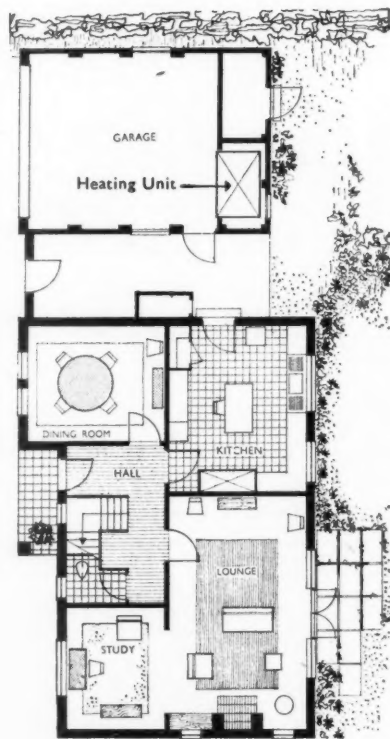
The automatic heating unit is housed in the garage, with ducts leading into the house. Small, unobtrusive grilles, set in the walls, circulate the warm air throughout the rooms.
