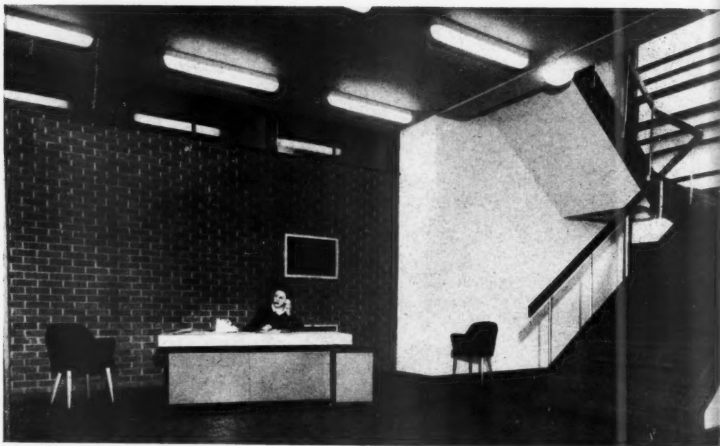
The entrance hall and inquiry desk. The staircase is in-situ concrete with a terrazzo finish.
