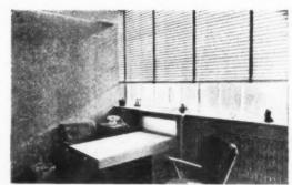
View of Director's Office: Insulated double-wall Compactite partitions faced with Etchwood; desk and fitments designed and constructed by Compactom.
