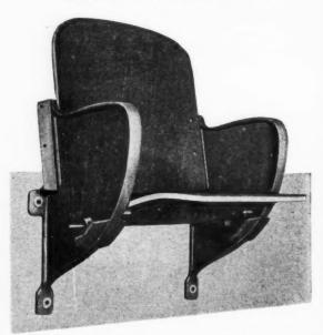
Modern styling. Seat and back made of laminated ply faced with rose coloured 'Formica'. Other surfaces finished pale grey. Solid fine cast seat standards, shaped to provide an integral armrest, have three point fixing to special channel grids set in the concrete risers. Chairs can be finished in any desired colours.
