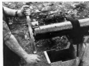
A special hand lathe is used for cutting joints on short lengths.
