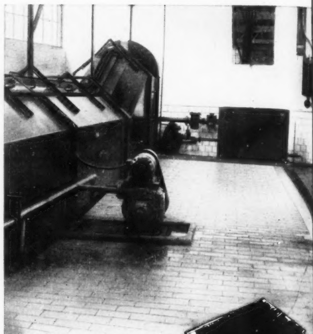
Resistant floor paving and dado adjacent to plastic lined and coated Fluxing Tunnel.
