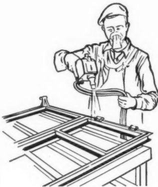
STAGE 2 Applying the zinc
