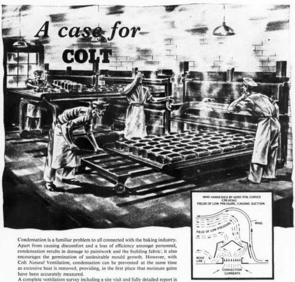
Above is a sectional view of the Colt SR type ventilator often used in bakeries. Without any of the disadvantages of noise, wear and tear, maintenance or running costs, one of these ventilators can provide continuous positive extract at a rate of 400,000 cubic feet per hour.
