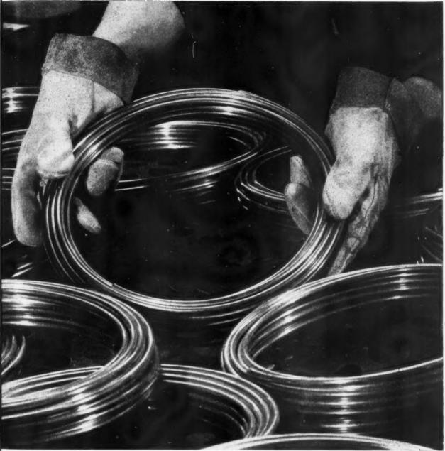
at of specialised production of coils for refrigerators.
