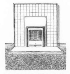
Fig. 2. Hearth type fire with horizontal radiants.
