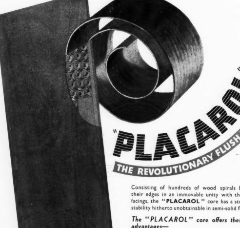
Consisting of hundreds of wood spirals bonded by their edges in an immovable unity with the plywood facings, the "PLACAROL" core has a strength and stability hitherto unobtainable in semi-solid flush doors.
