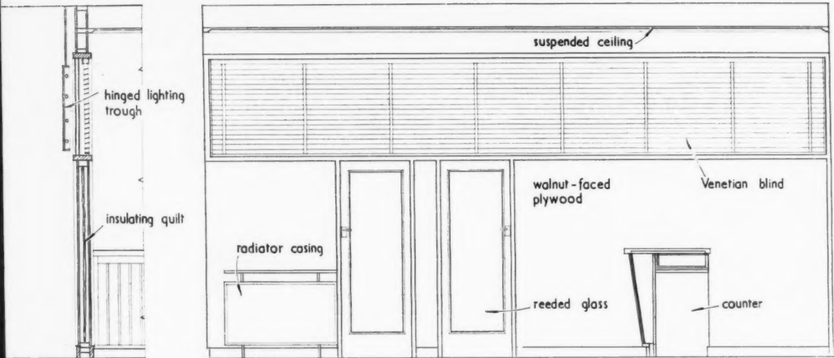
SECTION AND ELEVATION OF PARTITION. scale \frac{1}{4}'' = 1'-0''
