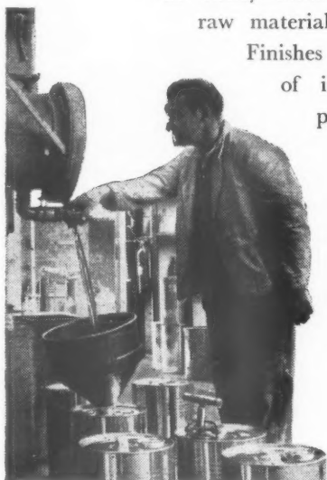
Filling from a mixing vat through visible measuring tanks.
