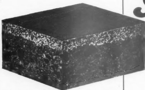
Section of a Stelcon Steel Clad Flag which shows clearly its great density.
