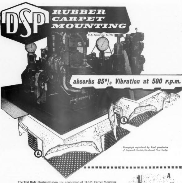
The Test Beds illustrated show the application of D.S.P. Carpet Mounting to Engine foundations providing isolation from the surrounding structure. The method of application of the Anti-Vibration carpet is decided by the vibration characteristics of the individual Engines.
