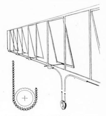
Fig. 6. Helical cable remote control window gearing.
