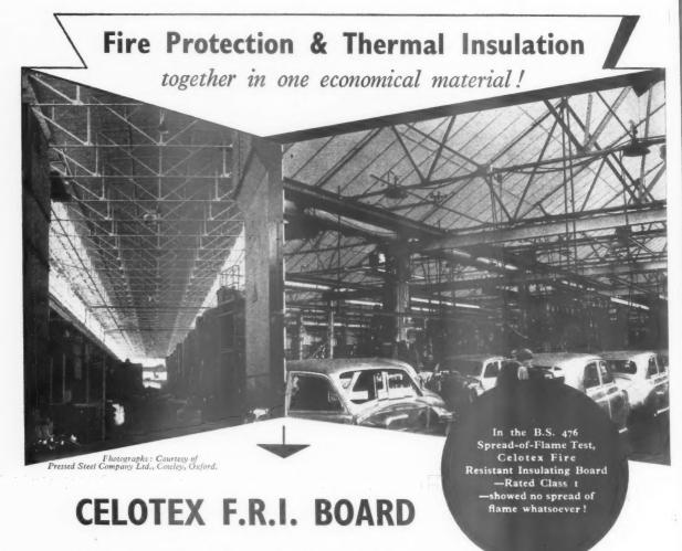
The world renowned thermal insulation of Celotex is now combined with the fire resistance of asbestos to form Celotex Fire Resistant Insulating Board. It's a core of tough, durable Celotex cane fibre insulation sheathed on both sides with asbestos felt, which, if required, can be easily decorated.
