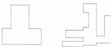
Fig. 1, two areas of 10,000 sq. ft. The enclosing wall area of (a) is 11,000 sq. ft., that of (b) 12,000 sq. ft.
