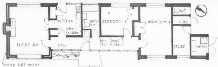
Ground floor plan [Scale: \frac{1}{4} " = 1' 0"]
