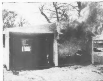
Striking demonstration of the ability of Albi-"R" to stop the spread of fire. The left-hand half of this wooden structure was coated inside with Albi-"R". Both sides fired simultaneously with a blowlamp.
