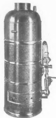
H.D. Industrial Multipoint. An instantaneous Heater in four sizes with capacities from 6 to 16 gallons per minute (raised 40° F. above cold). For Sports Pavilions, Kitchens and Automatic Dish Washing Machines where a continuous supply is required.
