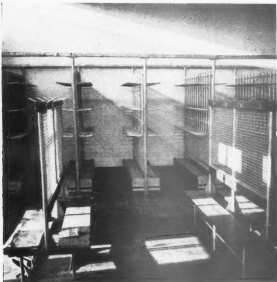
(11) Changing room. The racks in the background provide for the storage of each pupil's gymnasium clothing and towel. This was an early attempt at providing space for all the pupils' belongings; simpler methods are being examined.
