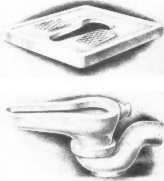
A squatting type w.c. suite, comprising white glazed, fireclay, tread plate with separate earthenware pan (which is, of course, placed beneath it) and loose "s" and "p" trap, vented.
