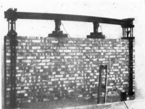
10' CLEAR SPAN. 11" CAVITY WALL CARRYING 11 TON TEST LOAD
