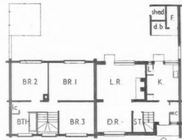
View 4. First and ground floor plans [Scale: \frac{1}{4} " = 1' 0"]
