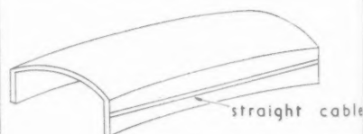
Right, Fig. 7. The position of prestressing cables in a barrel vault without edge beams compared with one with edge beams. Left, Fig. 8. Photograph of prestressing cables in the valley between two shells without an edge beam. Note the high degree of curvature which is possible, as indicated in Fig. 7. Right, Fig. 9. Barrel vault, arched in direction of span, so that prestressing cables can be straight. Below, Fig. 10. Bus garage at Sheffield, covered by thirty 97-ft. 6-in. long prestressed concrete shells, in 3 rows, designed on the principle illustrated in Fig. 9. (Sheffield City Architect's Dept. Consulting engineer, H.G. Cousins.)
