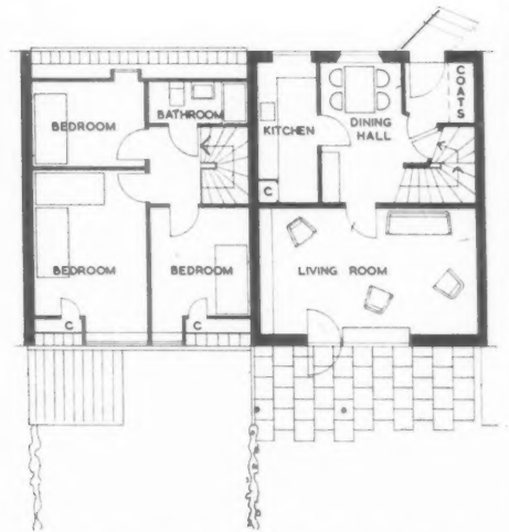
Ground and first floor plans of typical two-storey terrace houses [Scale: \frac{1}{4}" = 1' 0" ]
