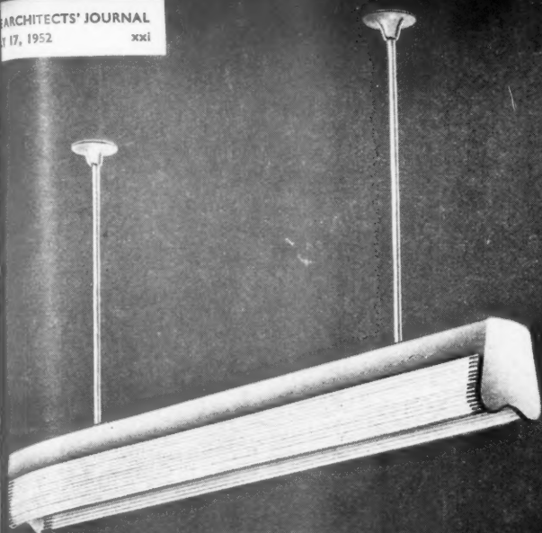
T416P Pendant. Type: diffused general with direct downward light. Finish: stove enamelled off-white. Perspex: 1 in. internal reeds. Lamps: two 4-ft. tubular fluorescent. Control gear: with starter switches only.
