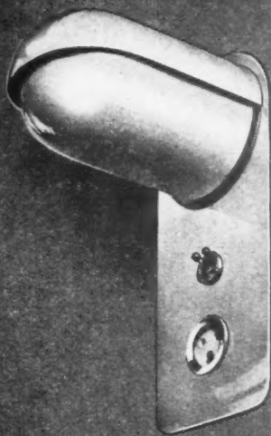
U.7H Flush. Bracket Recessed. Finishes: chromium and off-white. Glass: white flashed opal. Lamp: up to 60 watts. Socket: 2-amp 3-pin. Switches: 5-amp for lamp and socket.
