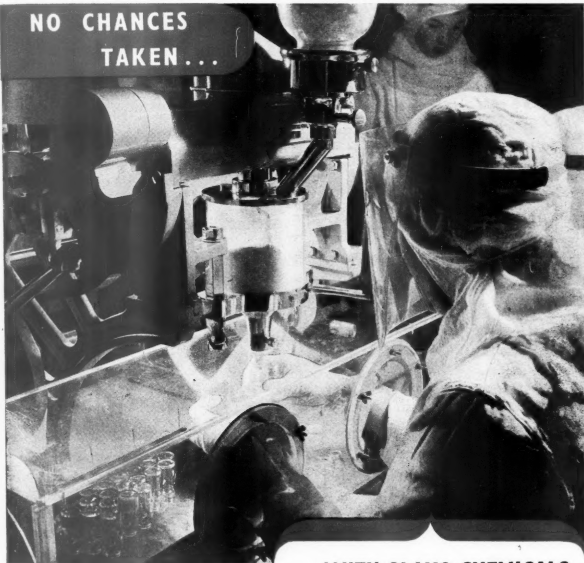
Filling vials with Streptomycin Glaxo in the Ampoule Department of Messrs. Glaxo Ltd.'s Ulverston Factory
