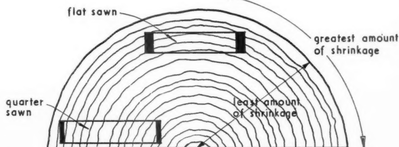
Fig. 1. Shrinkage of wood. Black parts indicate relative amount of shrinkage.
