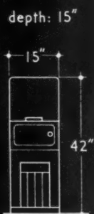
combined breakfast cooker and fire: 1 boiling burner and small oven
